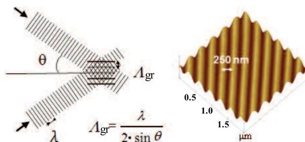
**Fig. 3** Formation of SRG on an azopolymer, as generated by two-beam interference irradiation. The grating pitch,  $\Lambda_{gr}$  is determined by the wavelength and the incident angle of the irradiated light. The figure on the right exhibits a topographical image as measured by AFM.
