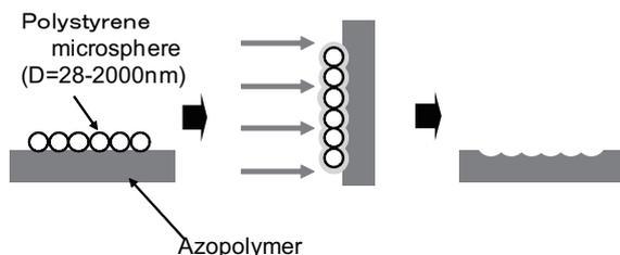
**Fig. 5** Schematic representation of a nanopatterning process formed by using microspheres as the near-field source, showing the alignment of the microspheres (left), light irradiation (center), and the elimination of the microspheres (right).
