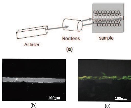
**Fig. 8** (a) Experimental setup for patterned immobilization using a linearly shaped laser beam. (b) Dark field optical image of immobilized polystyrene microspheres with diameters of 1  $\mu\text{m}$  on the surface of an azopolymer. (c) Fluorescence image of the immobilized  $\lambda$ -DNA molecules.<sup>(17)</sup>
