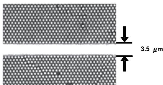
**Fig. 20** Area-selective photoimmobilized 2-D colloidal crystals (waveguide-type pattern).
