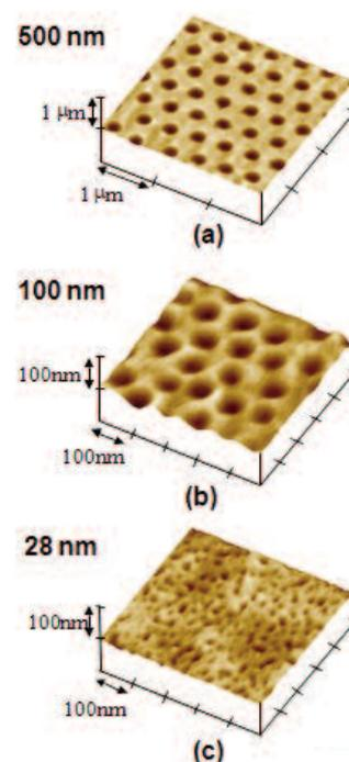
**Fig. 6** AFM images of nanopatterned structures formed on an azopolymer surface using microspheres with diameters of (a) 500 nm, (b) 100 nm, and (c) 28 nm, respectively.<sup>(19)</sup>
