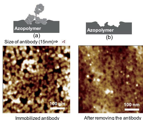
**Fig. 9** AFM images obtained from the photoimmobilization process. (a) The surface was observed after the photoimmobilization of immunoglobulin. The real-size immunoglobulin is shown. (b) The surface was observed after an elimination process using 2-wt% sodium dodecyl sulfate (SDS) solution.
