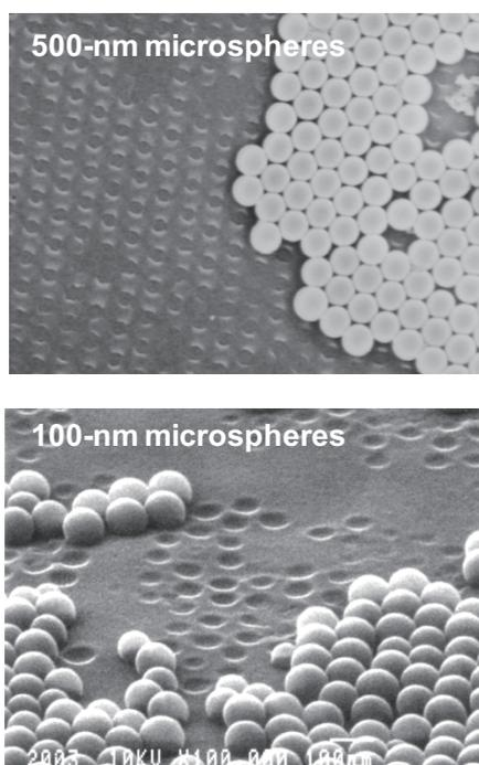
**Fig. 7** SEM images of nanopatterned structures formed on an azopolymer surface formed by using microspheres with diameters of 500 nm (top) and 100 nm (bottom), respectively. The microspheres remain partially.<sup>(29)</sup>
