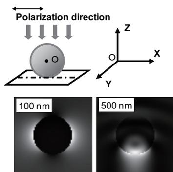
**Fig. 4** Calculated distribution of the optical intensity on the X-Z plane of the polystyrene microspheres, 100 nm (left) and 500 nm (right). The bright region indicates a relatively strong intensity.
