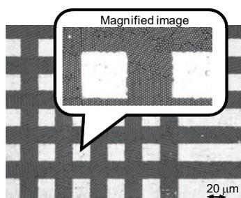
**Fig. 18** Microscope image of area-selective immobilized 1- $\mu\text{m}$  diameter polystyrene microspheres on the flat surface of an azobenzene-containing polymer film. The irradiated area was controlled by moving the sample stage.<sup>(35)</sup>
