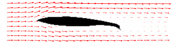
Fig. 3 Optimized results in lift maximization for Re = 100 with constrained drag force.
