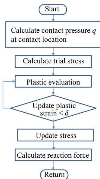
Fig. 3 Flowchart of the numerical algorithm for stress time integration using the proposed method.
