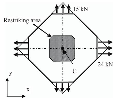
Fig. 4 Diagonal biaxial tensile test.
