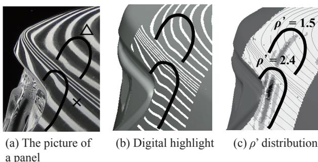
**Fig. 2** Comparison of a panel with the digital highlight inspection system.
