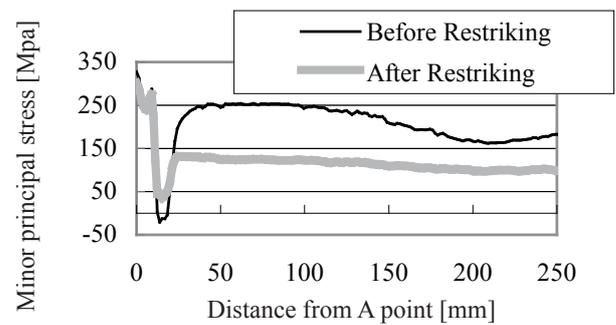
**Fig. 8** Minor principal stress distribution along A-A' section.
