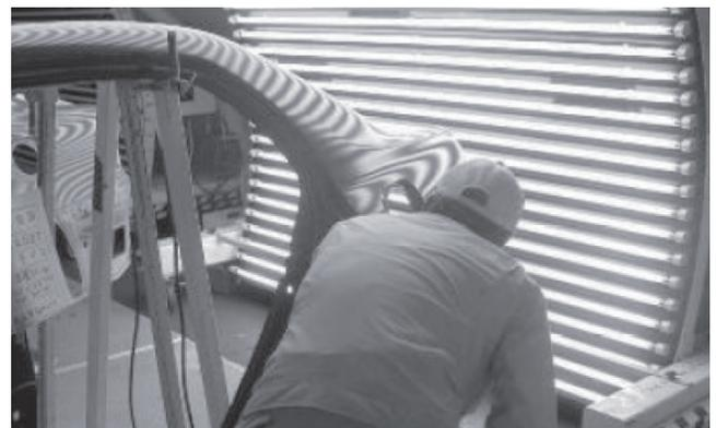
**Fig. 1** Surface quality inspection of a panel.
