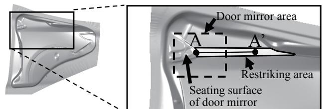
Fig. 6 Analysis model of a fender panel.
