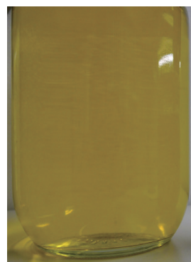
Fig. 7 Photograph of Pd nanocolloid prepared by laser ablation at the air-liquid interface.
