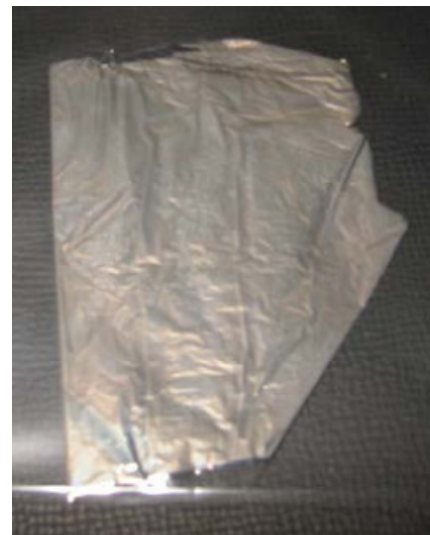
Fig. 8 Deuterated Pd/Ti thin films on polyethylene film.
