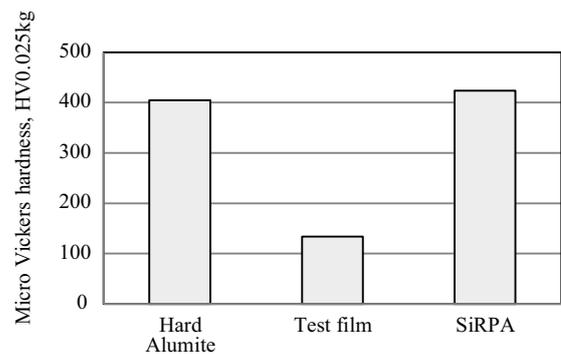
Fig. 9 Comparison of hardness of different films.
