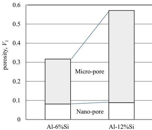
Fig. 7 Porosity of aluminum alloy films for different Si concentrations.
