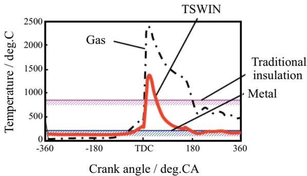
**Fig. 1** Gas and combustion chamber wall temperatures as functions of crank angle.
