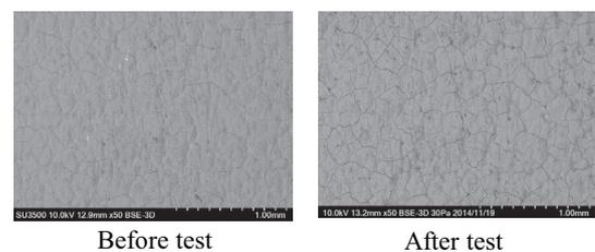
**Fig. 16** SEM images of SiRPA surface before and after engine test.
