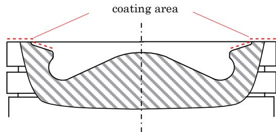
**Fig. 15** Schematic of piston region coated with SiRPA.
