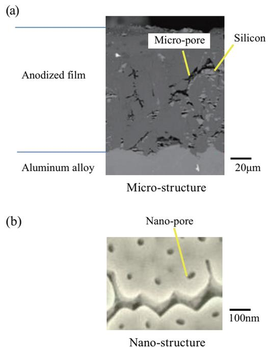
**Fig. 3** Structure of porous anodized aluminum employed in TSWIN technique.
