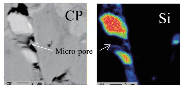
**Fig. 12** Si distribution around micro-pores.
