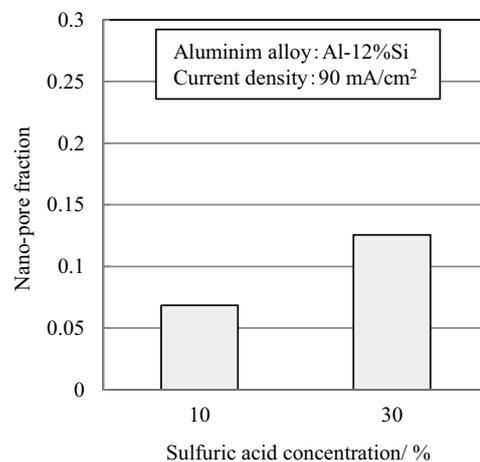
**Fig. 4** Fraction of nano-pores in anodized aluminum films for different sulfuric acid concentrations.
