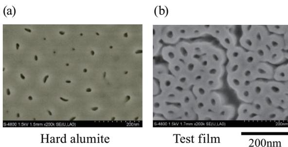
**Fig. 10** SEM images of nano-structure of anodized films.
