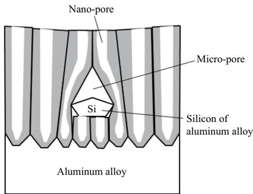
Fig. 6 Schematic diagram of anodized film on aluminum alloy.
