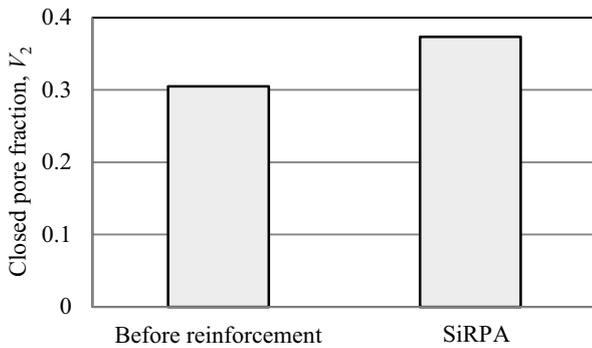
**Fig. 13** Closed pore fraction before and after silica reinforcement.
