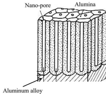
**Fig. 2** Structure of porous anodized aluminum.<sup>(6)</sup>
