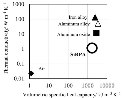
**Fig. 14** Thermophysical properties of various materials.
