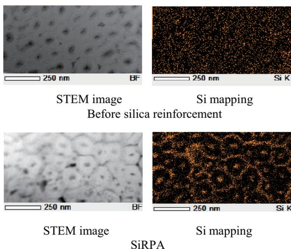
**Fig. 11** Si distribution in anodized film.
