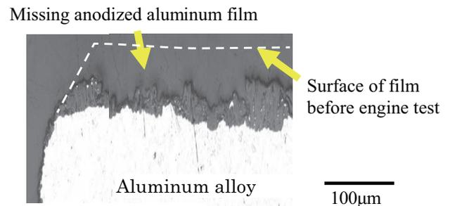
Fig. 8 Cross-sectional micrograph of anodized aluminum film following engine test.
