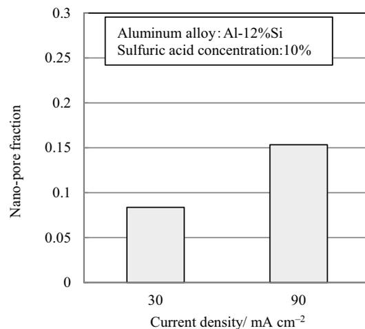
**Fig. 5** Fraction of nano-pores in anodized aluminum films for different current densities.
