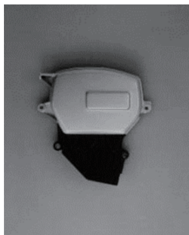
Fig. 1 Timing belt cover for an automobile engine made from NCH.
