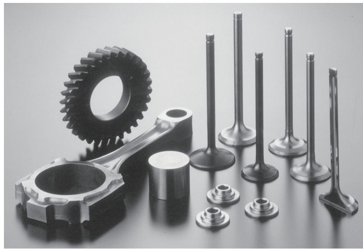
Fig. 42 Prototype automotive parts made of TiB/Ti-MMC produced by the developed B/E process: spur gear, connecting rod, valve lifter, valve retainer, and hollow valve, etc.
