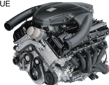
Fig. 2 Appearance of Lexus LFA and its NA 4.8-liter V10 1LR-GUE engine.
