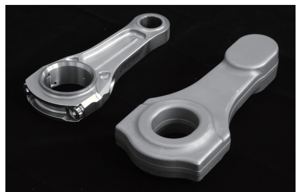
Fig. 4 Titanium alloy (SP-700) connecting rod for Toyota F1 engine (left) machined from hot forged preform (right).
