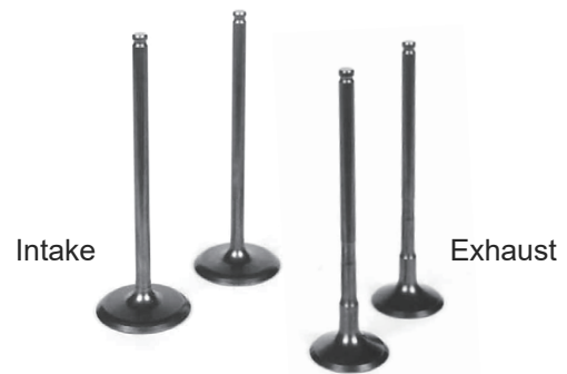
Fig. 1 The first mass-produced car in the world to feature TiB/Ti-MMC engine valves.
