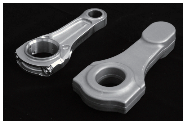
Fig. 4 Titanium alloy (SP-700) connecting rod for Toyota F1 engine (left) machined from hot forged preform (right).
