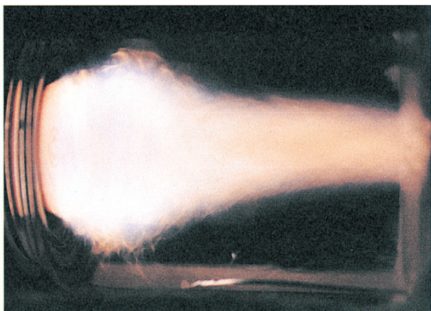
(a) Spray combustion in TPPL-1 combustion chamber
